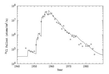
**Figure 16.** The <sup>36</sup>Cl bomb pulse in an ice core from Dye 3, Greenland. The solid line is the result of a box-model calculation (after Synal *et al* 1990).
