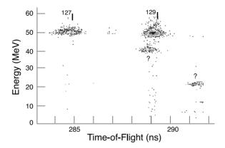
**Figure 5.** An energy versus time-of-flight spectrum obtained with the Chalk River detection system showing the clear separation of <sup>129</sup>I from other ion species. <sup>127</sup>I and <sup>129</sup>I are separated by 4.5 ns. A few <sup>128,130</sup>Te counts are visible between the iodine peaks. Peaks labelled '?' have not been identified. (From Koslowsky *et al* 1997.)
