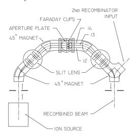
Figure 3. The recombinator injection system used by the AMS systems based on the Mk II Tandetrons.
