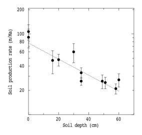
**Figure 13.** Soil production rates (calculated from *in situ* produced cosmogenic <sup>10</sup>Be and <sup>26</sup>Al in bedrock samples) versus soil depth for a series of sites in Tennessee Valley, Marin County, California (after Heimsath *et al* 1997).
