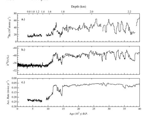
**Figure 14.** (a) The  $^{10}$ Be concentration in the Greenland Ice Sheet Project 2 (GISP2) ice core (Finkel and Nishiizumi 1997). (b)  $\delta^{18}$ O in the GISP2 core (Grootes et~al~1993). (c) Ice accumulation rate (Cuffey and Clow 1997). The bottom axis indicates the GISP2 timescale and the top axis is in terms of depth. The scales for  $\delta^{18}$ O and accumulation rate have been inverted for ease of comparison with  $^{10}$ Be. (From Finkel and Nishiizumi 1997.)
