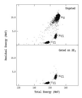
**Figure 9.** Bi-dimensional plot of residual energy versus total energy showing the separation of 154 MeV  $^{36}$ Cl and  $^{36}$ S ions. The lower plot was obtained after applying a gate on the  $\Delta E_3$  signal which accepted chlorine, but not sulfur, ions. The  $^{36}$ Cl/Cl ratio of the sample was  $430 \times 10^{-15}$ .
