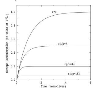
**Figure 11.** The surface concentration of a cosmogenic isotope in rock as a function of time and for different erosion rates. For  $^{36}$ Cl, one mean life is 430 ka, and  $P/\lambda$  at sea level and high latitude is  $1.3 \times 10^7$  atoms g<sup>-1</sup>.
