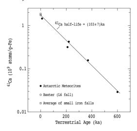
**Figure 18.** Determination of the half-life of <sup>41</sup>Ca from the relative concentrations of <sup>41</sup>Ca and <sup>36</sup>Cl in Antarctic meteorites with a range of terrestrial ages (from Klein *et al* 1991).
