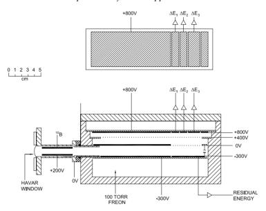
**Figure 7.** The <sup>10</sup>Be detector used at the Australian National University. It incorporates the stopping of <sup>10</sup>B and the measurement of the residual energy of <sup>10</sup>Be within the same gas volume.
