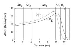
**Figure 8.** Energy loss as a function of distance into a gasionization counter for 154 MeV <sup>36</sup>Cl and <sup>36</sup>S ions. The positions of the anode electrodes of the detector shown in figure 4 are indicated.
