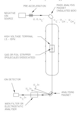
**Figure 1.** The essential features of an AMS system. The first magnet is shown as transmitting mass-14 negative ions. It is also set periodically to transmit mass-12 and mass-13 ions, in which cases the accelerated ions are detected in the off-axis cups after the analysing magnet.
