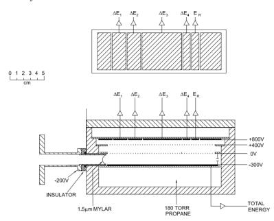
**Figure 4.** A cross section through the multi-element ionization chamber used at the Australian National University for <sup>36</sup>Cl, <sup>14</sup>C and <sup>26</sup>Al detection. The upper panel shows a plan view of the anode electrode.
