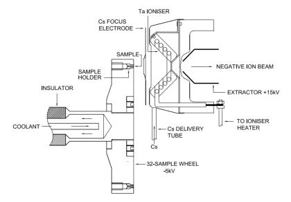
**Figure 2.** The basic components of a modern (NEC MC-SNICS) high intensity negative-ion source. The ionizer is at local ground potential, and the Cs focus electrode at a voltage intermediate between the ionizer and wheel.
