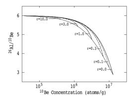
**Figure 12.** Plot of  $^{26}$ Al/ $^{10}$ Be ratio versus  $^{10}$ Be concentration for quartz exposed at the earth's surface. The upper solid curve is for zero erosion, and a series of curves for progressively higher rates of erosion (in mm ka $^{-1}$ ) are also shown. The lower solid curve is the locus of the end points of all such curves.
